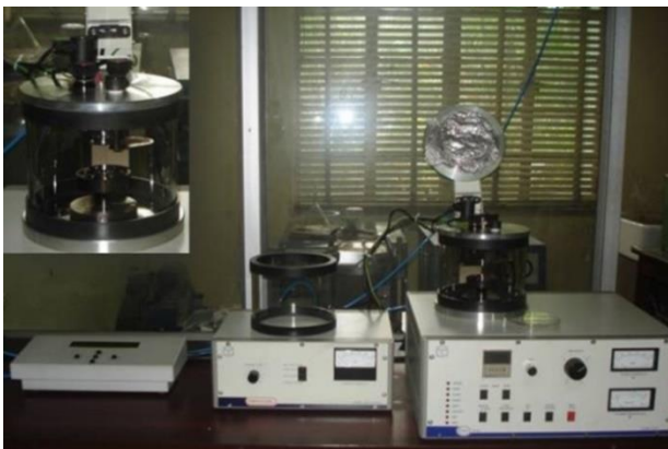
Fig. 5: Gold-sputtering machine (IB-2 ION COATER). Inset picture shows enlarged view of the sputtering chamber
