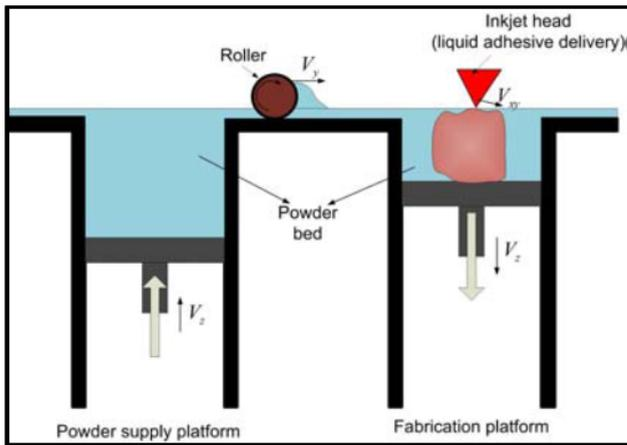
Fig. 3: Schematic diagram of Inkjet-based system
