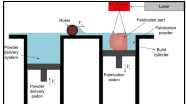
Fig. 4: Schematic diagram of selective laser sintering
